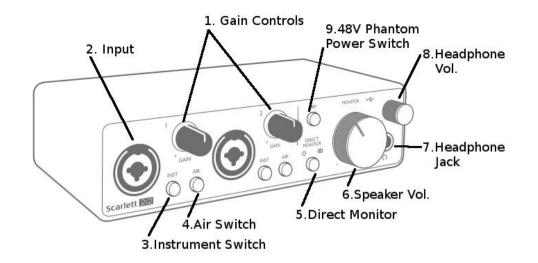
We use these dials to control the amount of **gain** being received by the interface from the cassette deck. If our gain is too high then the sound is clipped, which means the waveform gets cut off at the top and bottom. This will result in the inaccurate capture of data from the tape.
